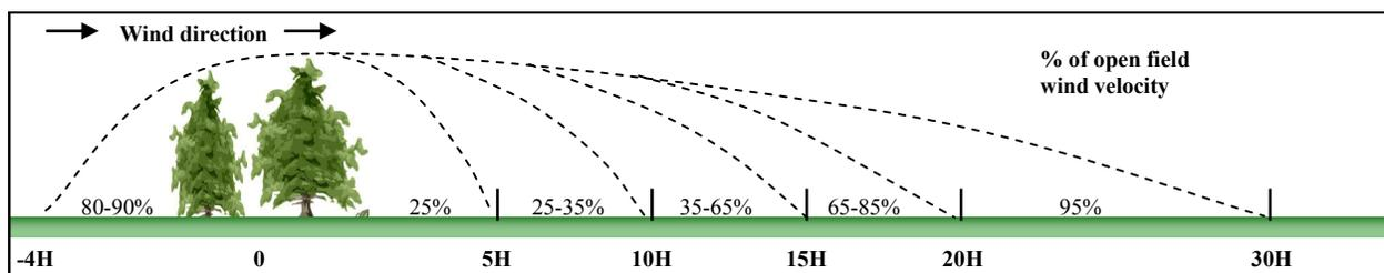
Figure 2. Multi-Row wind barrier, 60-80% density.
