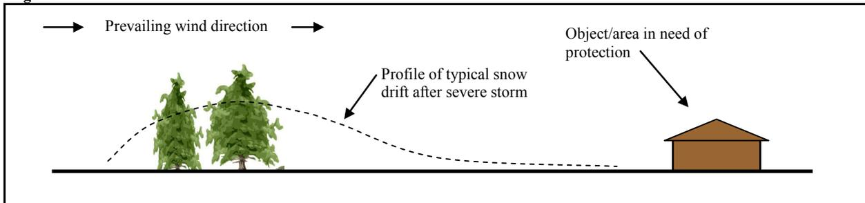
Basic windbreak consisting of two rows of conifer trees
